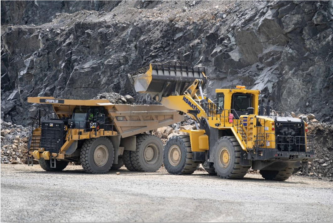
A Komatsu WA800 loader and a Caterpillar 777G haul truck work to bring shot rock to the primary crusher at H&K's Birdsboro Quarry located in Birdsboro, PA.
